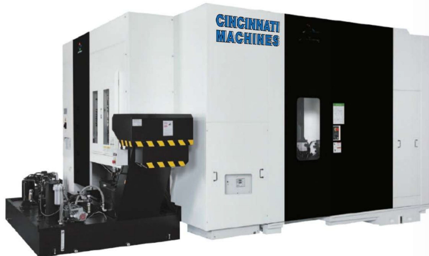
(Photo shows HS-630i with optional scraper roller type chip conveyor.)
