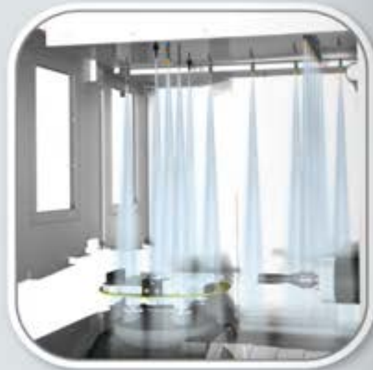
14 Nozzles Coolant Shower
