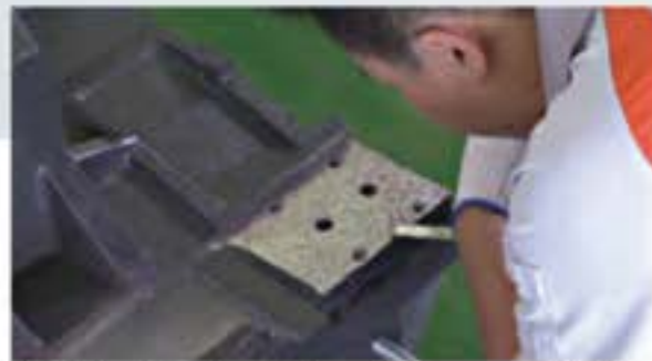
100% Hand-Scraping for Geometry Accuracy and Rigidity
