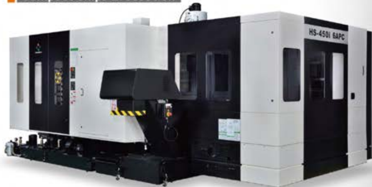
Photo shows HS-450I 6APC with optional scraper type chip conveyor
