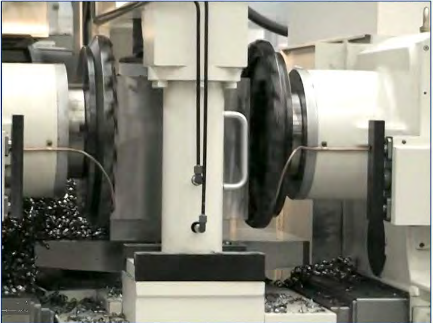
45° index table provides 4-corner chamfer milling
