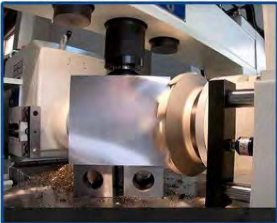
45° index table provides 4-corner chamfer milling
