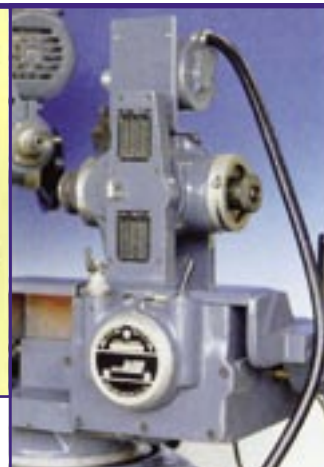
Spiral mechanism generates infinitely variable leads
