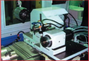
Swivel A&B Axes plus Twin Grinding Heads allow Multiple Grinding Jobs in One Setup
