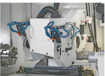
3 Spindles (2 OD 1 ID) that are indexed via B-Axis under CNC Control provide Optimum User Ease of use and performance characteristics.
