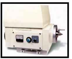
The Heavy-duty Meehanite cast workhead features an 8 piece precision angular contact bearing set and state-of-the-art electronic variable speed spindle drive. The combination live and dead type spindle allows for quick change from chuck to live center setup or vice-versa. The workhead swivels 90° counterclockwise and 30° clockwise for vesatility.
